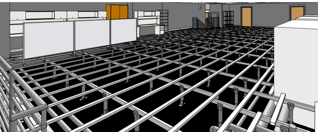
Iso Floor supporting 745 PSF (36.5 kN/m 2 ) of electrical equipment for a major technology company in Arizona.
