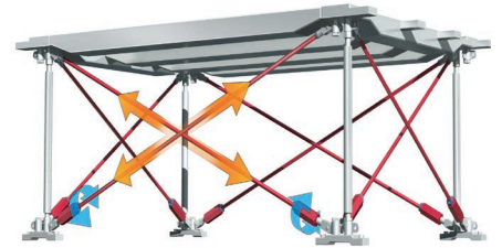
Model 1.0 is for floor heights up to 919 mm (36 inches) having pre-torque cross braces to achieve required stiffness at high floor heights
